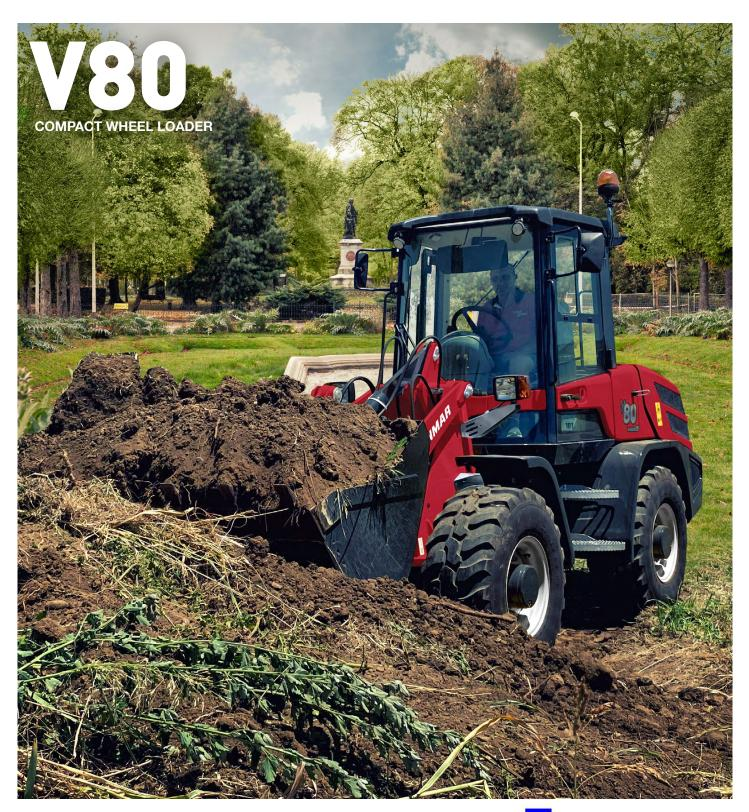
Operating weight Net Power Bucket capacity Steering 4 900 kg 46,2 kW (63 HP) 0,8 – 1,2 m<sup>3</sup> Articulated steering
